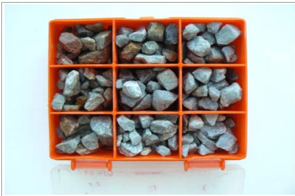
Figure 10-1: Drill Cuttings for Logging. Red Fragments indicate oxidation, Grey Fragments indicate Sulphide Material
